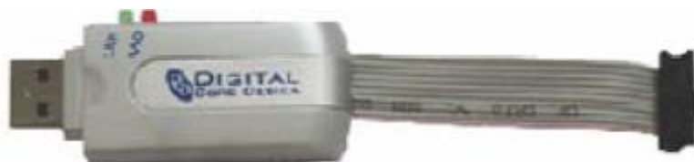
Figure 18. DoCD HAD2 Debugger Module
